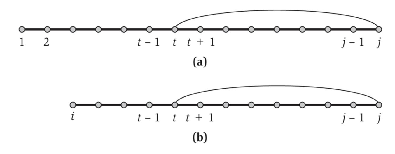
**Figure 6.15** Schematic views of the dynamic programming recurrence using (a) one variable, and (b) two variables.
