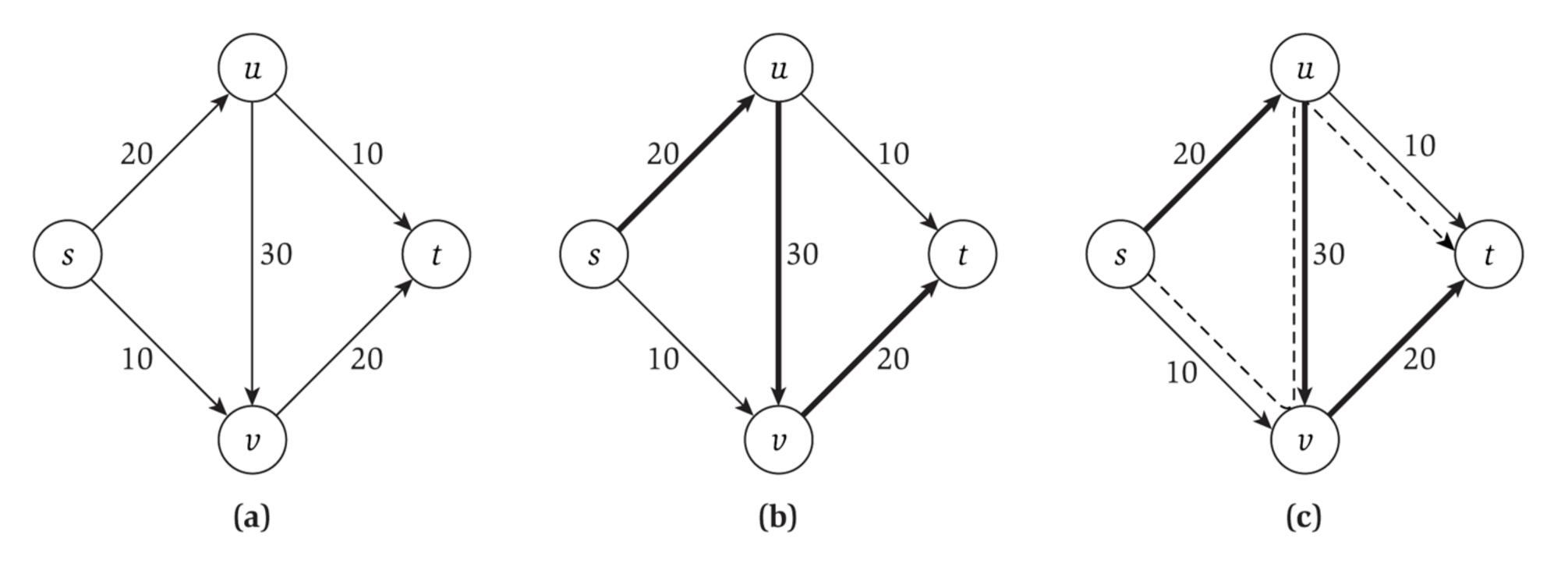
**Figure 7.3** (a) The network of Figure 7.2. (b) Pushing 20 units of flow along the path s, u, v, t. (c) The new kind of augmenting path using the edge (u, v) backward.
